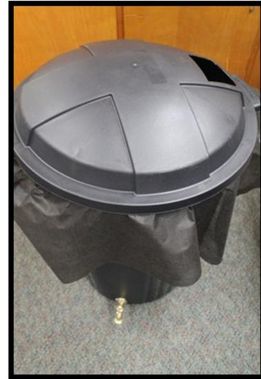
7. Cut a piece of landscaping fabric to sit over the top of your rain barrel, putting the lid over the top of it to secure it. This will create a barrier that prevents mosquitoes and other pests from getting in your rain barrel water.
