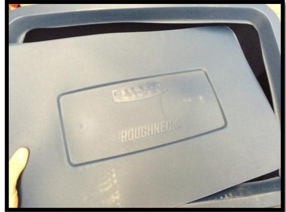
1. Cut out the center of the container lid using the box knife. Cut a small rounded notch in one corner to fit the size of the PVC pipe. Save this piece for later use.
