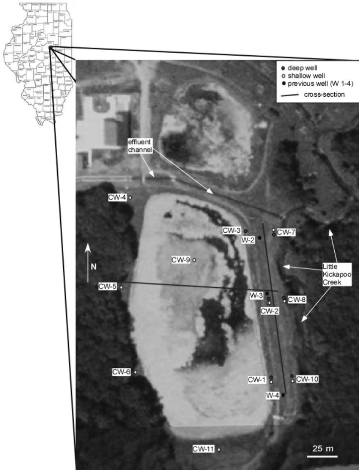
**Figure 1:** BNWRD study site highlighting the constructed wetlands. Well locations and the position of Little Kickapoo Creek are identified. Note three wells, CW-9, CW-6, and CW-11, were not used in this study and Wells W1, W2, W3, and W4 are no longer present.
